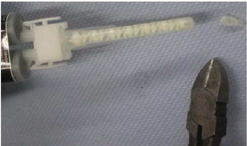
Fig. 55: Attach adapter, unscrew mixing tube, shorten mixing tube
