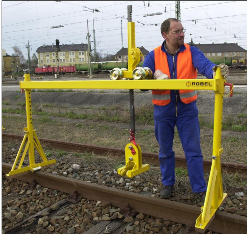
Fig. 26: Manual movement along the rail
